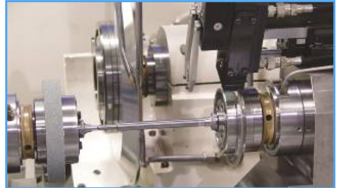
Inside PPG – grinding between centers
